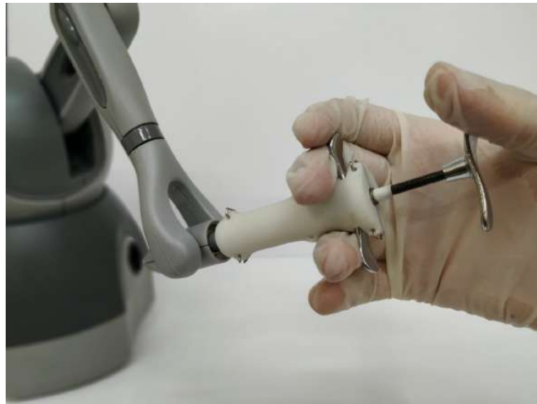
Figure 7 – Modified haptic device by replacing the device stylus with a real syringe.
