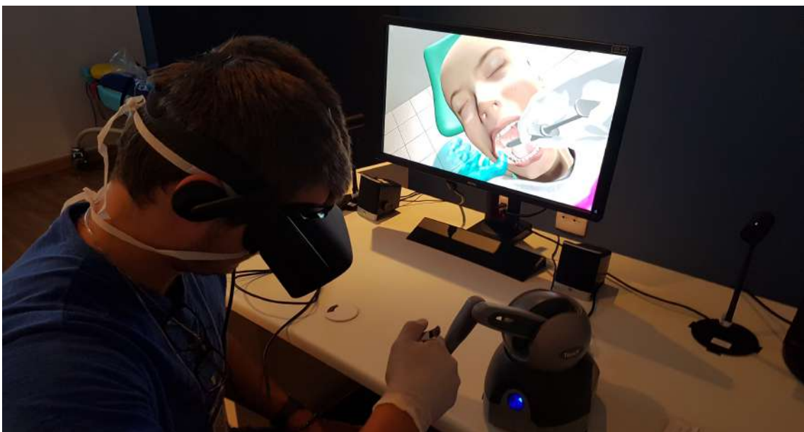
Figure 4 – The VIDA Odonto ® haptic VR simulator.
